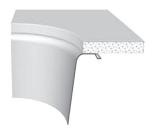
Check if the cut fits the Inox sink and place it in the desired position. At every 10 to 15cm of the Inox sink glue the bearing screws.
