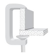
In case of Kerrock sheets which contain metal particles (Metal, Luminaco S and Marble effect), the appearance of the surface and edge of the sheet differ, so make sure the edge is not visible when making joints. There are two ways for doing that:
