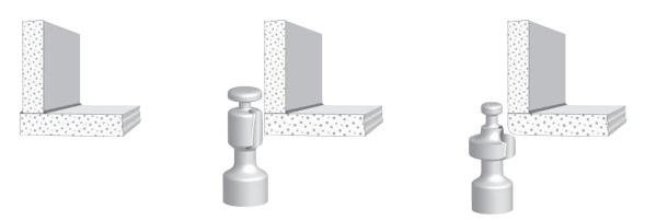
In the case of the groove method, makea groove on the back side of the kitchen counter reaching up to the 2/3 of the counter deep, which is as wide as the thickness of the glued piece. The patch is glued into the grooved part.
