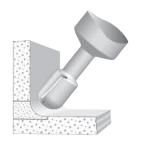
The processed piece is then cut leaving 2-3mm of edge, which is glued on the countertop, where we have previously made a groove 2-3mm deep and 25mm wide.
