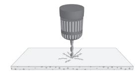
If screwing joining in the Kerrock surface is required, we must insert a brass or PVC cork. Observe work conditions which apply for glass or other more fragile materials. The borehole must be approx. 10% bigger than the screw's diameter. We must also insert a spacer between the Kerrock surface and a screw and the second material with screw joints.
